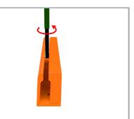
To adjust the mounting carrier, unlock the latch via operating tool (5.5 mm blade) and move the clamping slide to the required width by rotating the tool.
