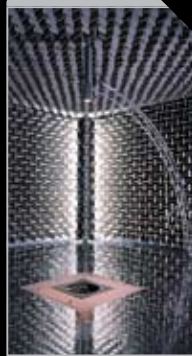
Sound testing in anechoic chamber
