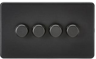
Push on/push off control. Advanced trailing edge type dimmer suitable for dimming all types of lamps both resistive and inductive. Minimum capacity: 5W dimmable LED or 10W incandescent. Maximum capacity: 150W dimmable LED or 200W incandescent. Suitable for mains lighting, low voltage lighting and LED lighting (for compatibility please check with lamp manufacturer).
