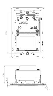
Dual voltage shaver sockets come complete with transformer and isolated mains supply which is safe and suitable for bathroom use.
