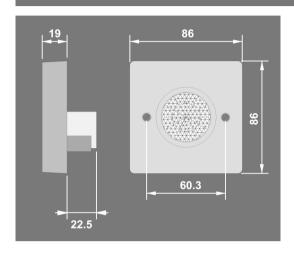
The SPIR-F/C presence detector switches are designed to provide automatic control of lighting, heating or ventilation loads. They detect movement using a PIR sensor and turn the load on. When an area is no longer occupied the load will switch off after an adjustable time out period.
