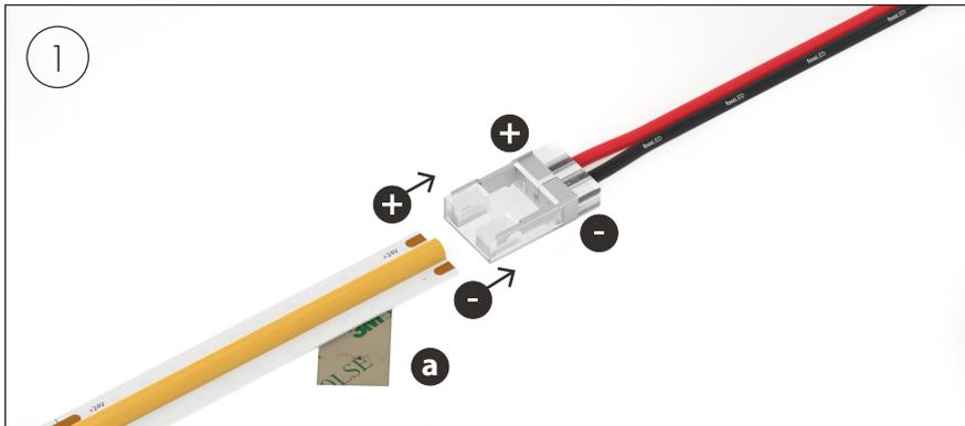
**a** Peel back the adhesive tape leaving a sufficient amount of bare strip to insert into the clip. Make sure you peel back the tape and accompanying adhesive layer leaving this to re-apply once the connection is complete.
