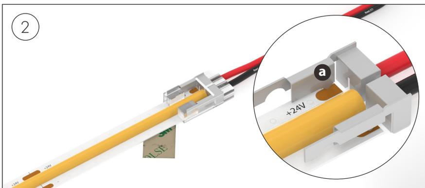
**a** Insert the LED Strip into the corresponding terminals ensuring the strip is fitted correctly so that the copper pads line up with the clip connector teeth.
