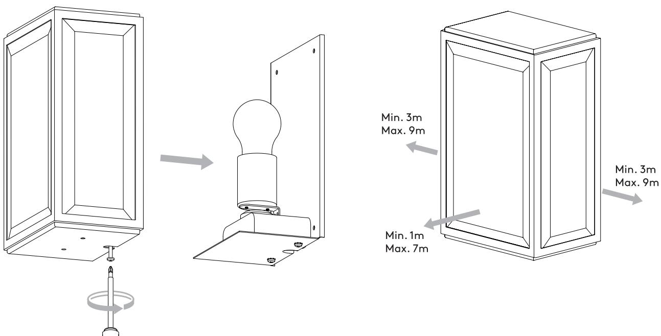
**GB** NOTE: Do not adjust the three setting knobs to excess. Do not attempt to rotate beyond the rotation-stops. Multiple products must be mounted more than 4 meters apart to avoid interference.
