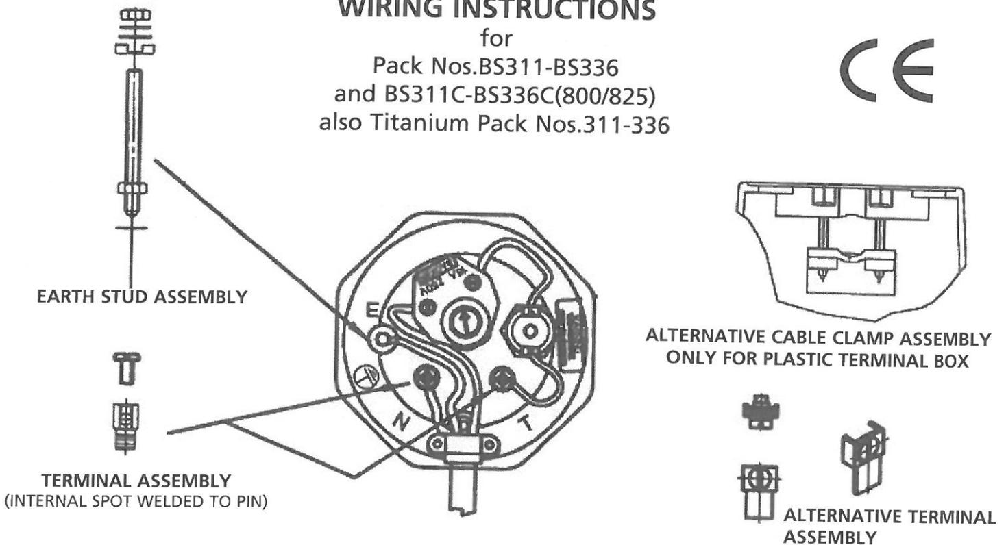
This heater is designed to take Backer BT-65° thermostats and fitted with a manual reset cutout.
